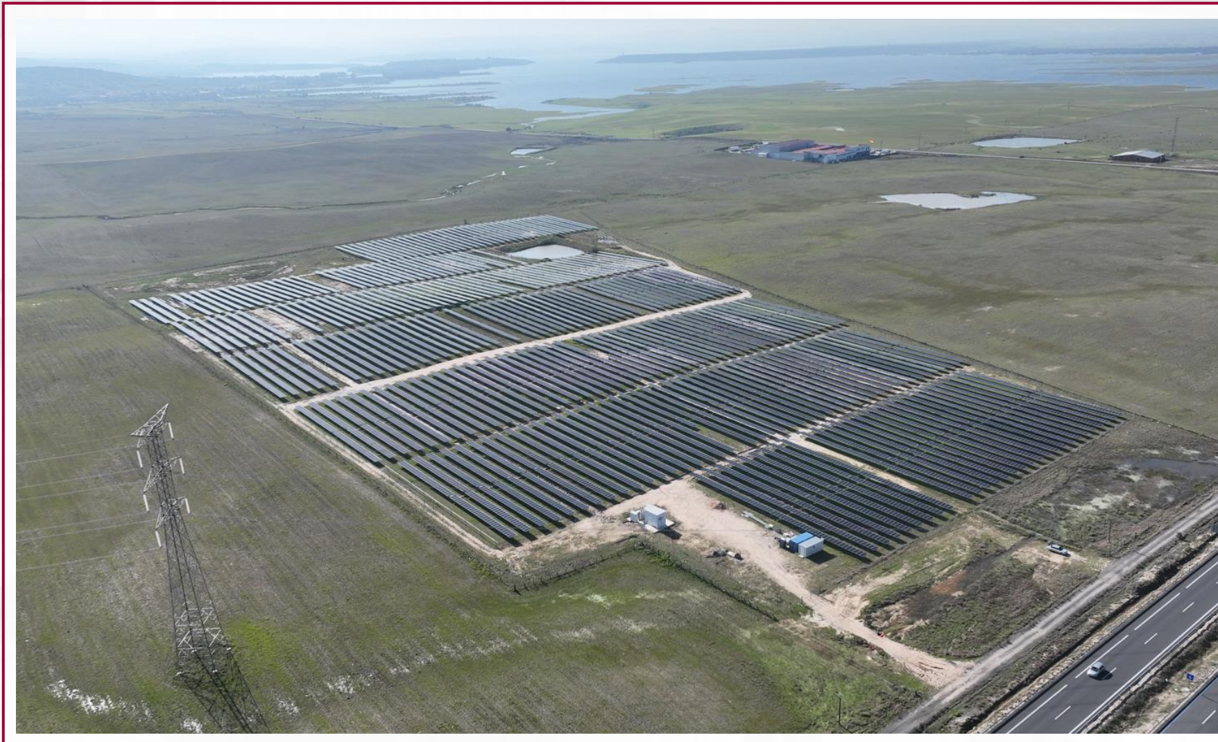
Tormillo III y IV photovoltaic generation plant in Huesca 2.4 MW capacity 5.2 K modular solar panels
